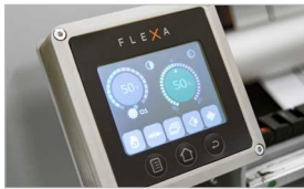
Automatic vertical alignment control panel
