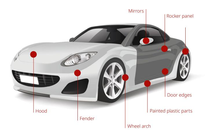
When using application fluid it may take 3-5 days, depending on film thickness, ambient temperature and humidity, until the residual moisture has fully evaporated and the cloudiness has disappeared and the final appearance has evolved.
